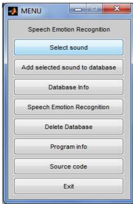
Figure 1. Graphical User Interface (GUI) of the Neural Network
