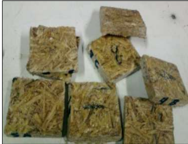
Figure 7. Test Specimen for Internal Bond Strength Test
