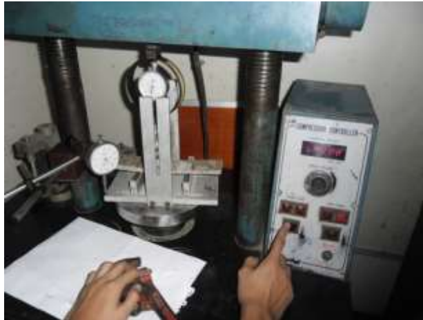
Figure 4. Modulus of Rupture Test Set – Up
