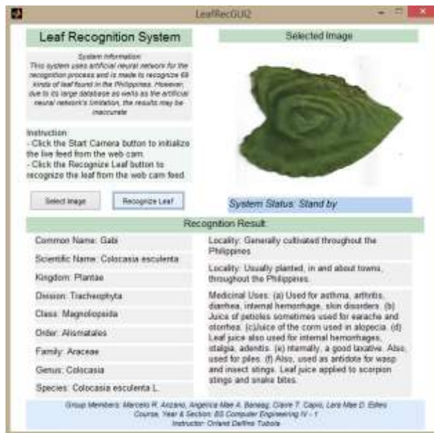
Figure 9. Recognition of Gabi leaf using the neural network with 75 neurons trained with the database containing more than 100 leaves.
